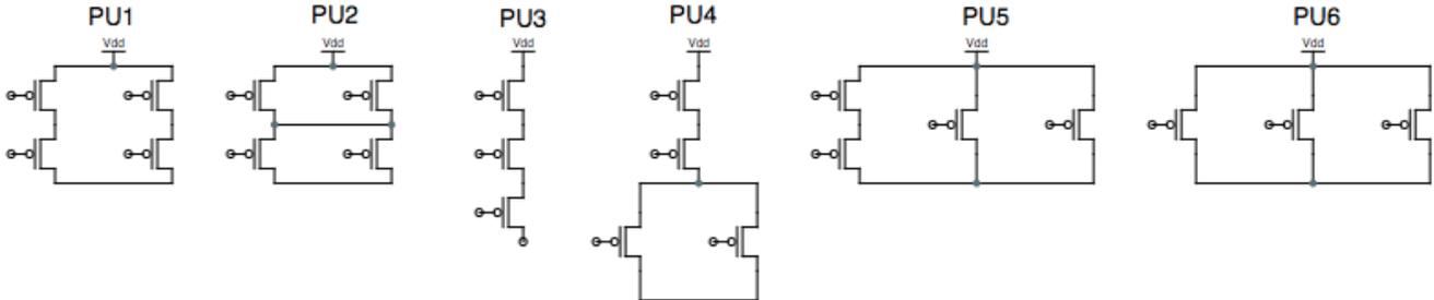
You can connect one of the inputs (A, B, C, or D) or a constant (GND, or VDD) to each pFET, allowing these pullups to be used in various ways to build gates with various numbers of inputs. Your goal, however, is to select the pullup that uses the minimum number of active transistors for each of the gates you are designing (i.e., a pFET that is never on is *not active*).
